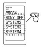
11 Press the Label Select button or other button on the Commander of which the function you want to program as a step. (To change the labels, press the SCROLL button repeatedly.)
